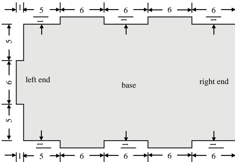
Glue the five panels together to form the drawer. The right end doesn't have any finger joints: it's glued directly onto the ends of the panels.
