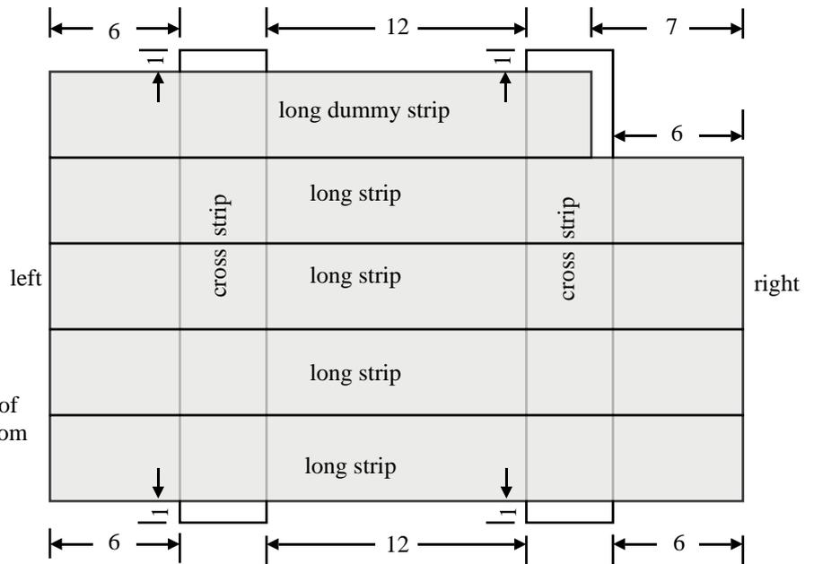
Glue three long strips onto the shorter cross strips in the positions shown.
