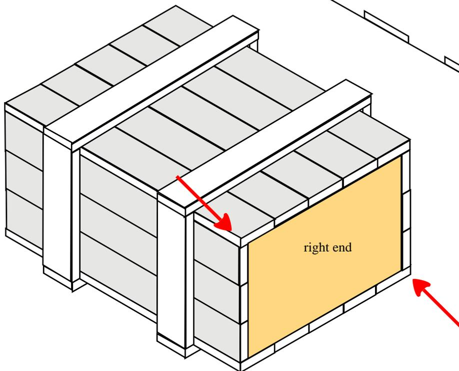
Push the drawer into the box. The short dummy strips should just fit under the longer cross sliders, hiding the inner ends. To open the drawer, grip the top and bottom corners of the box shown by the red arrows, and pull.
