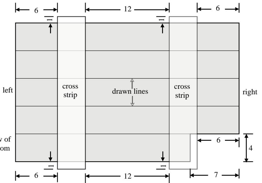
Glue the shorter cross strips onto the front and back panels in the positions shown.
