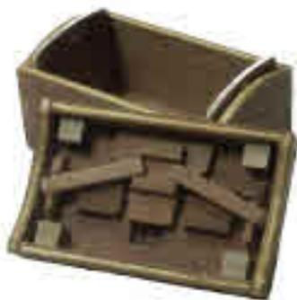
For the finish, I stained and varnished the box, and painted the top panels black, before gluing the top panels to the sliders. The inside was lined with green baize.
